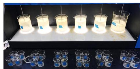
**Image 3.** A jar test set-up for the Bosque water with 50mL beakers for samples.
